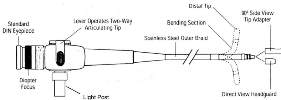
users can adjust the lens set to their particular vision prescription and use the Hawkeye Blue flexible borescope without glasses. All Hawkeye Blue Flexible borescope eyepieces are of standard DIN design and therefore compatible with standard eyepiece attachments such as camera couplers.
