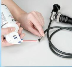
Dampen a cotton swab with Hawkeye lens cleaner, isopropyl alcohol or acetone. Clean the surface gently, taking care not to scratch it.
